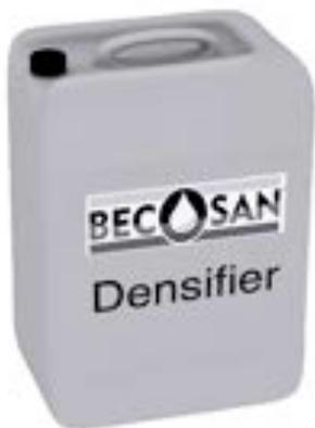
BECOSAN® Densifier, is a hardener and dust proofer for concrete surfaces, and is a water based solution which penetrate and react with free lime or calcium hydroxide within the concrete surface. The chemical reaction produces a denser concrete surface, which reduces abrasion wear plus reduction in dust formation and increased resistance to chemicals.
